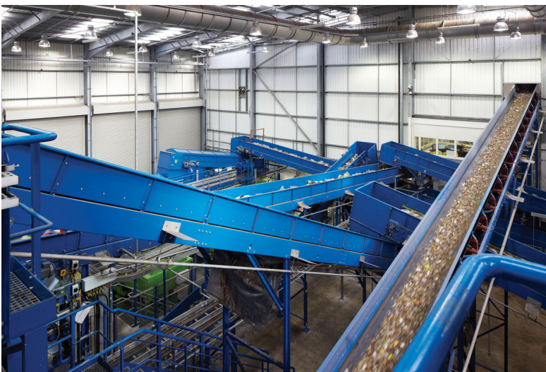
Plate 2 : Typical modern MRF process conveyors
